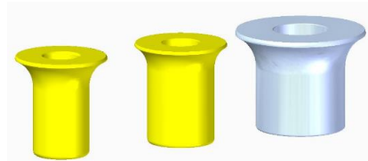
Figure 255, Comparison of the proposed new smaller tubular rivets with a standard size tubular rivet.
