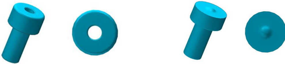
Figure 270, Stage 1 – hollow die (left), stage 2 – raised die (right)
