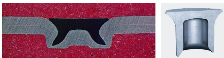
Figure 18, Successful riveting of very thin 0.75mm to 0.75mm aluminium for a car door using sharp tip A-rivet.
