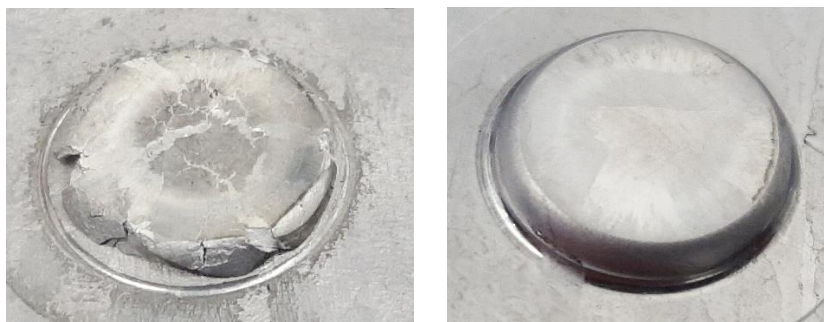
Figure 40, Example of button cracking in an aluminium casting being solved by heat treating the casting. (Briskham 2019)
