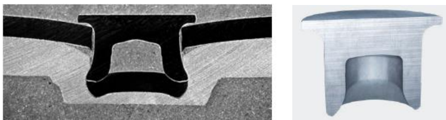
Figure 20, Picture of the latest rivet design called the BG-rivet, developed for joining UHSS to aluminium
