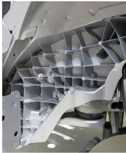
Figure 4, Cadillac CT6 car body showing rivbonding of sheet/cast/extruded aluminium with sheet steel. (Source Visnic 2019)
