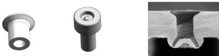
Figure 12, Initial Semi-tubular SPR design with square rivet tips
