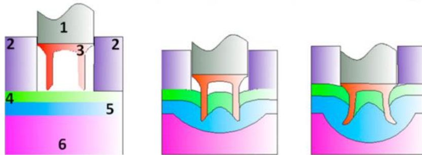
Figure 57, Schematic diagram of hydro forming SPR process (Haque, 2017).
