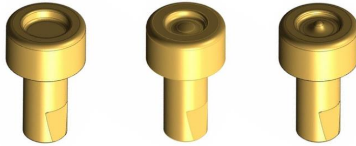
Figure 28, From left to right, 3D dwg of DG, DP and DZ type dies.
