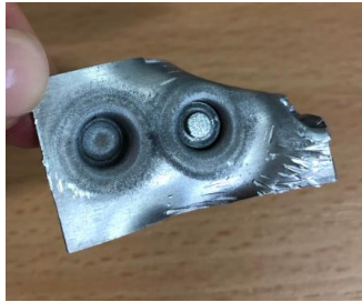
Figure 179, Rivet removed from joint to show wear of the coating
