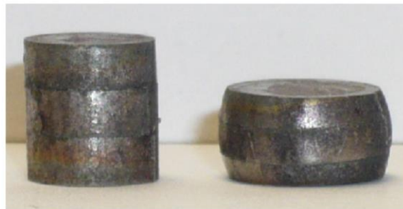
Figure 107, Bulging behaviour in stack compression test with glued stacks. (Hochholdinger, 2009)
