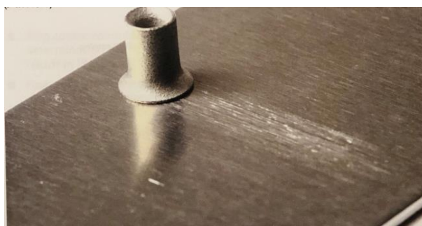
Figure 138, Sample rivet measured using translational sliding test
