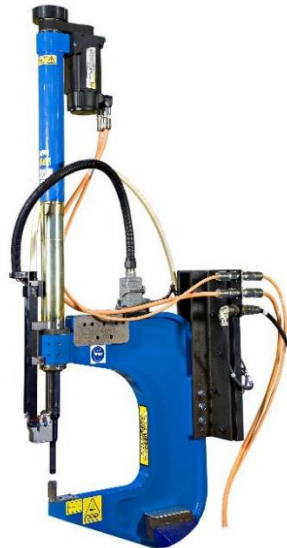
Figure 32, Standard robot mounted Henrob servo tool for blow feed rivet supply
