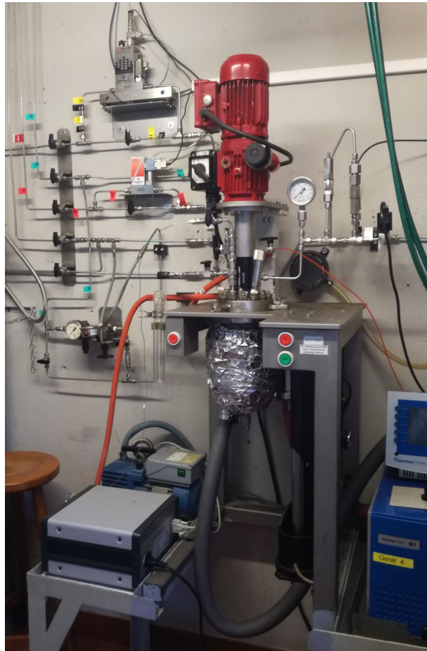
Fig. 5 High-pressure reactor system at the JKU Linz (Credits: Patricia Pappenreiter, JKU Linz)
