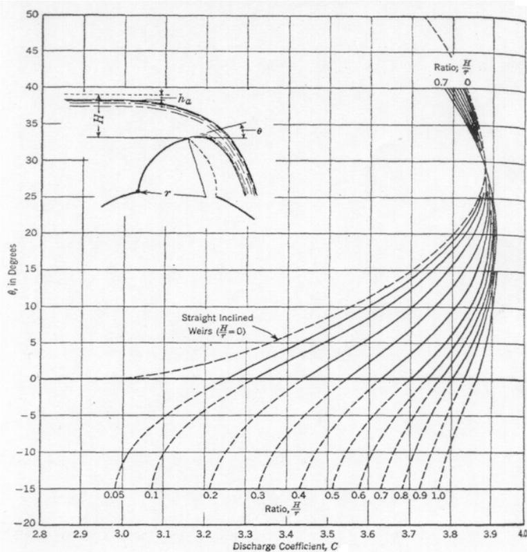
Figure 1. Discharge coefficient  $C$  [ $\text{ft}^{1/2} \cdot \text{s}^{-1}$ ] (Bradley 1954)
