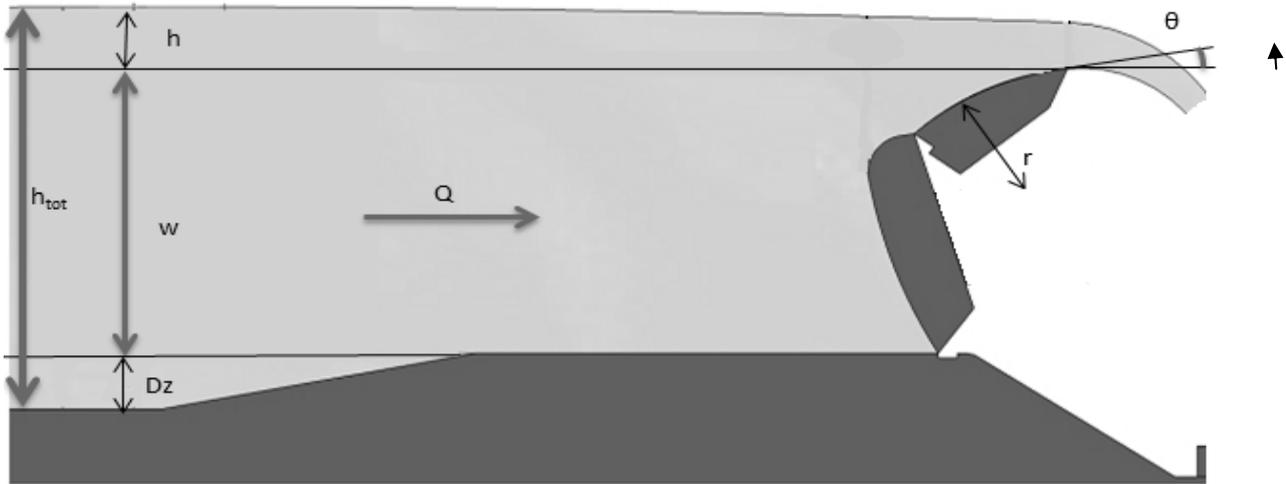
Figure 8. Sketch of the experimental set-up with geometrical parameters
