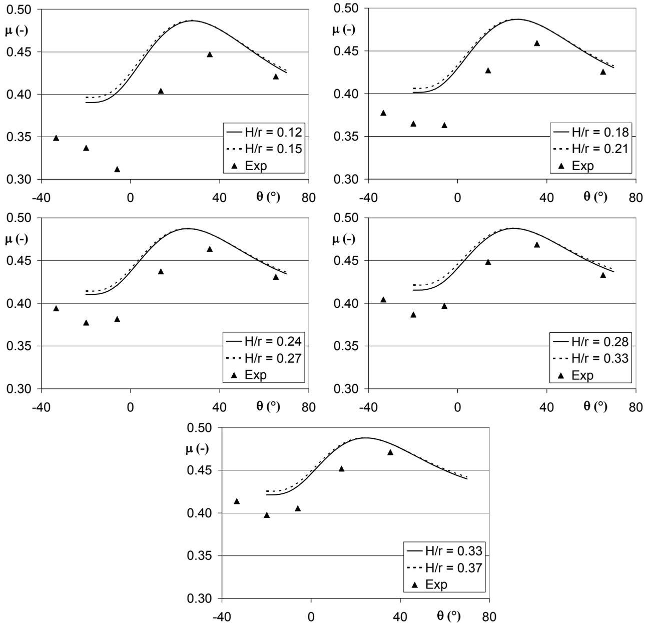
Figure 9. Discharge coefficient vs.  $\theta$  (angle between the horizontal and the tangent to the downstream lip of the gate). For  $H/r > 0.33$  the measurement was not possible at  $\theta = 65.24^\circ$  due to too high upstream level compared to the channel design.
