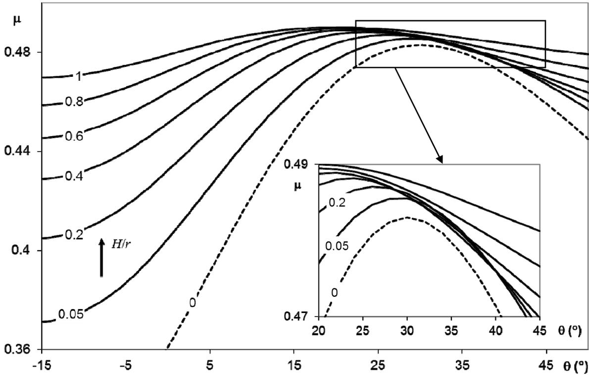
Figure 3. Discharge coefficient following Sinniger and Hager (1989)
