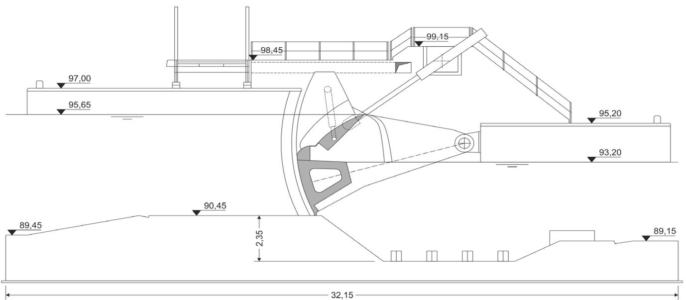
Figure 6. Transversal view of the gates in place on the Meuse River with upstream and downstream channel
