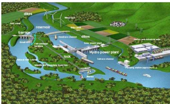
Figure 1. Typical low-head development scheme.
