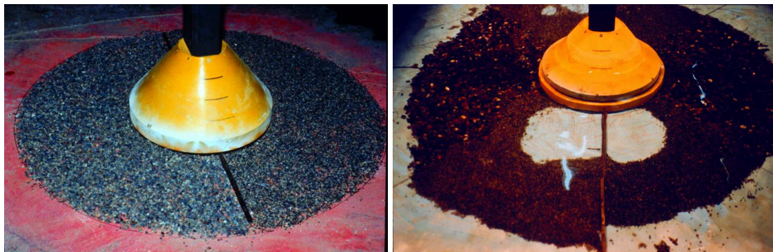
Figure 7 – Tracer Mat Around Model Approach Pier Before and After Test
