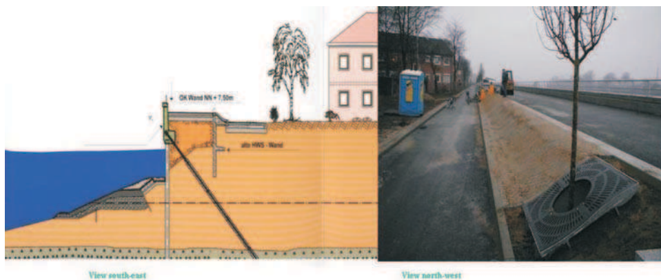
Fig. 10: Public storm surge protection wall ‘Köhlfleet’, Hamburg (graphics and photo: HPA, 2002)
