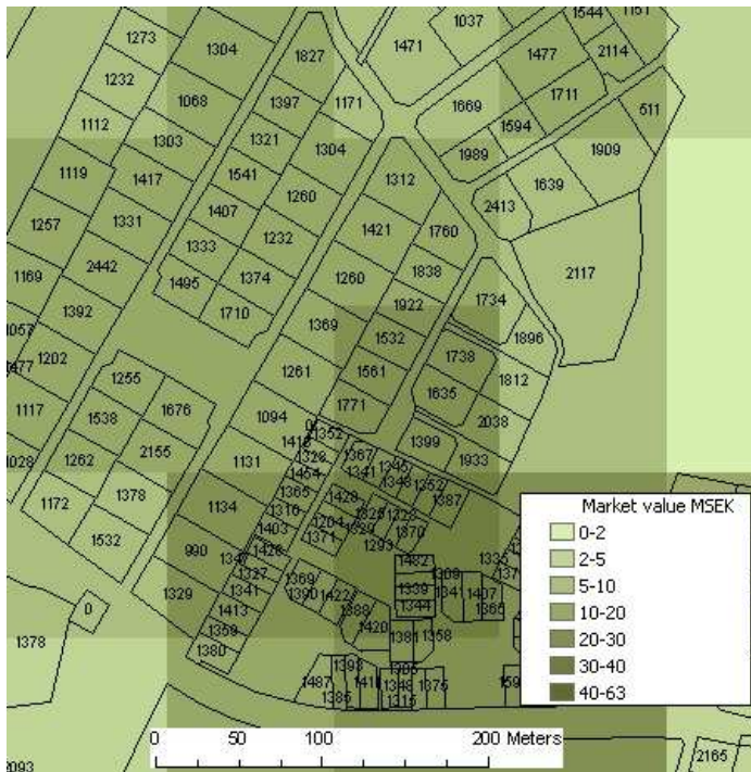
Figure 3. A real property map with taxation values in kSEK (shown in figure) and purchase price / taxation value ratios are the inputs for calculating market values. Market values are shown as raster data with the cell colour showing the value in MSEK of each 100 by 100 m cell. 1 SEK \approx 0.1 €.
