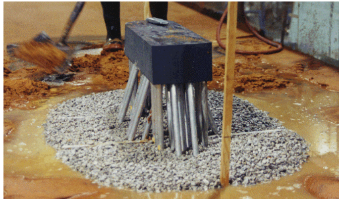
Figure 2 – Standard Pier and Scour Pad in Test Flume
