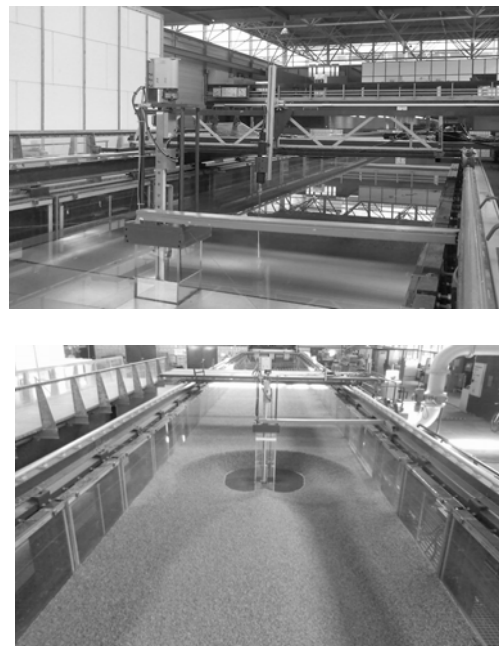
Figure 2. Experimental set-up with plane (upper) and scoured bed (lower).
