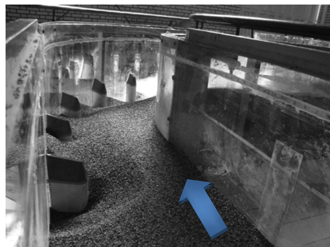
Figure 5 Bendway weirs at 4L spacing and Froude number equal to 0.3(looking downstream)
