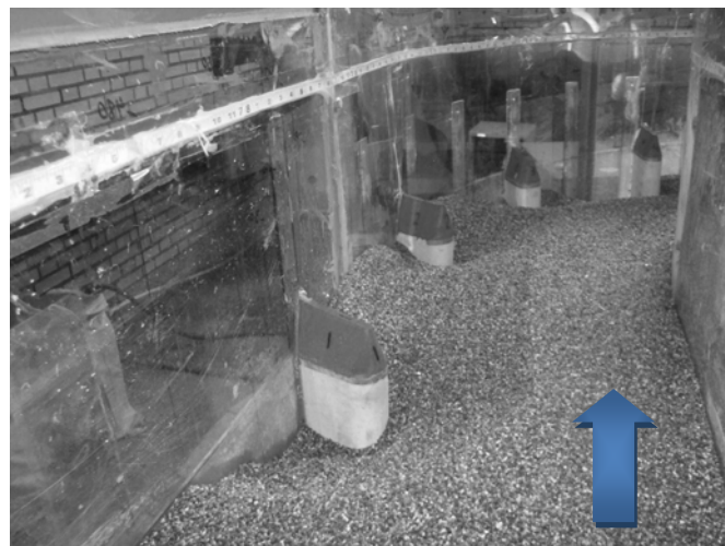
Figure 4 Bendway weirs at 5L spacing and Froude number equal to 0.3(looking downstream)
