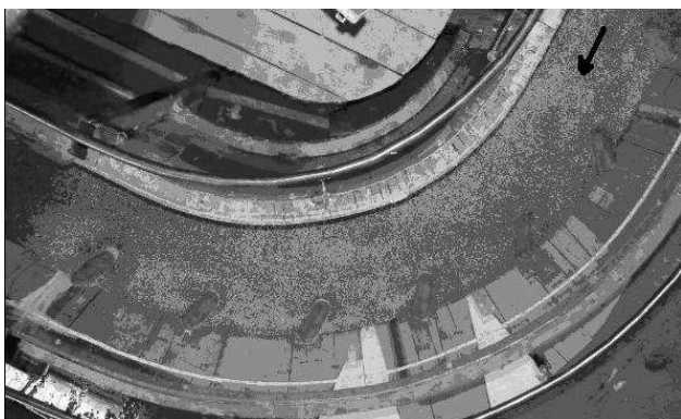
Figure 2. View of 90° bend flume with weirs installed.
