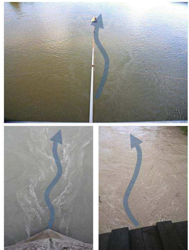
Figure 7: Observation of bridge-piers at the Danube/Voest-bridge (top), Inn-river in Innsbruck (lower-left) and Hall (lower right)
