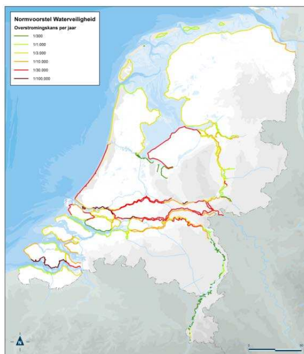
Figure 1: Proposed new safety standards for flood defences in the Netherlands, in the form of target failure probabilities for a system ( Delta Program, 2014 )
