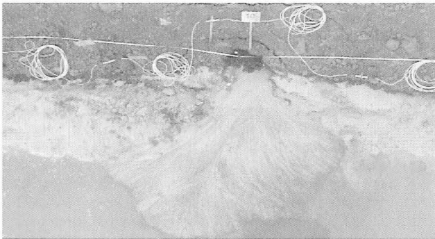
Figure 10: Widening of channel has reached the downstream side, resulting in an increase of sand transport, in this case followed by deformation
