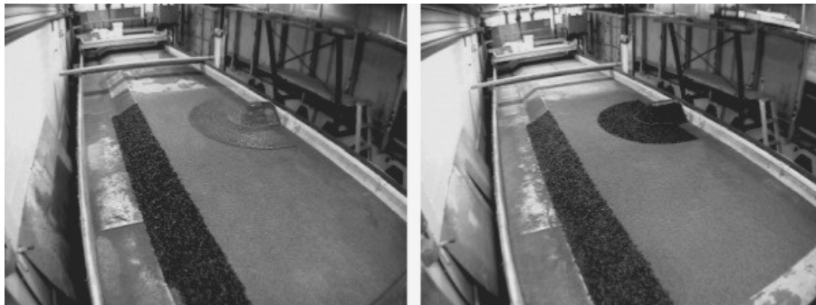
Figure 2. Experimental set-up of a 0.6-m-long abutment protected by a 0.5-m-wide apron situated on a 1.6-m-wide flood plain. Left; CTB apron. Right; riprap apron.
