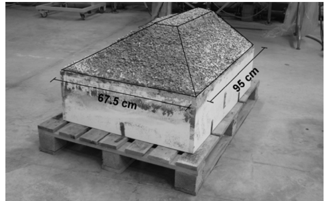
Figure 6. View of the rigid groynes.
