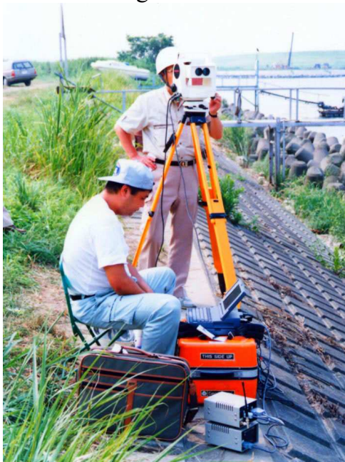
Photo 5 - Measurement of RC boat's location by total station
