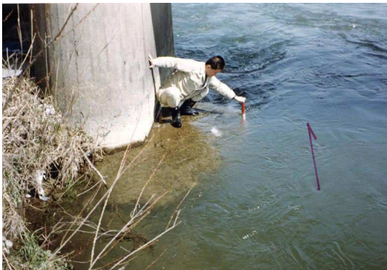
Photo 1 - Conventional investigation technique for scour from a footing
