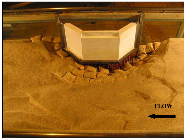
Figure 5. The scour hole developed for the geobag configuration shown in Figure 4.
