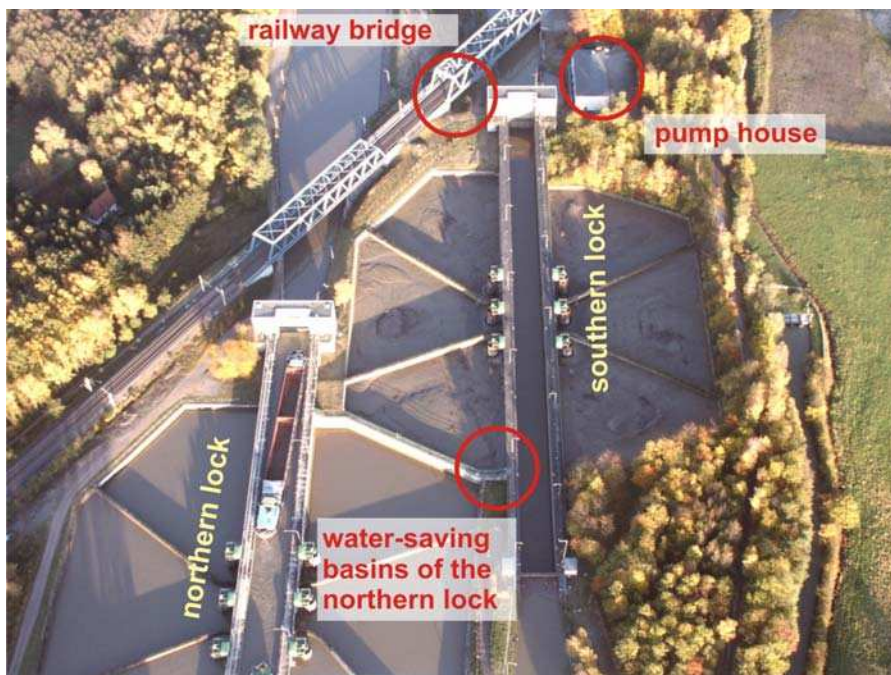
Figure 4: Location of the neighbouring structures
