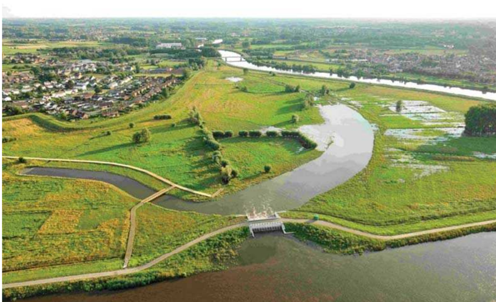
Figure 1 - Bergenmeersen: Flood control area (FCA) with controlled reduced tide (CRT) along the Scheldt estuary, Belgium (picture: www.sigmaplan.be )
