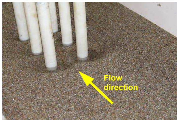
Figure 4. Scour hole at equilibrium stage for 2x3 pier group: G/D = 2 ; D = 22 mm; h = 4.7 cm.
