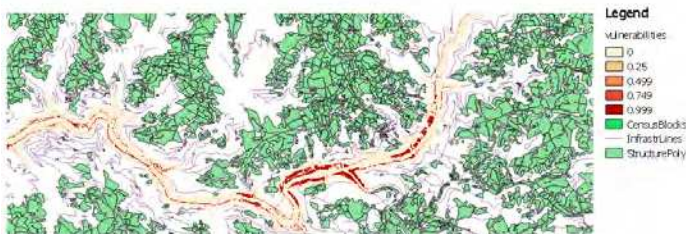
Figure 14 Vulnerabilities map at the downstream area for total instantaneous dam failures scenario
