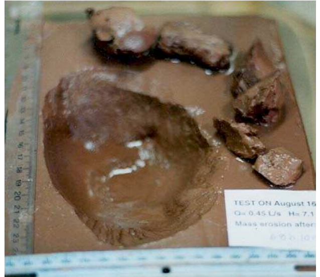
Figure 3. Larger chunks removed during an experiment with H=65 mm, d=8 mm, and a U_o=8.95 m/s over 68 h of testing
