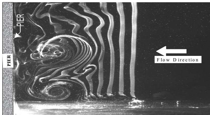
Figure 1. Photo of Visualized Flow in Front of a Bridge Pier
