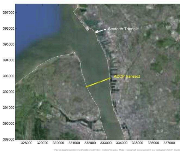
Figure 6. Locations of the proposed Water Injection Dredging (Seaforth Triangle) and the sediment flux measurements (ADCP transect) in the Mersey Narrows.
