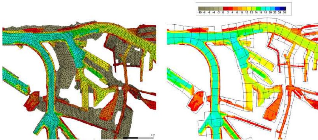
Fig. 11 Bathymetry of Hamburg harbor using classical unstructured grid (left) and subgrid technique (right)
