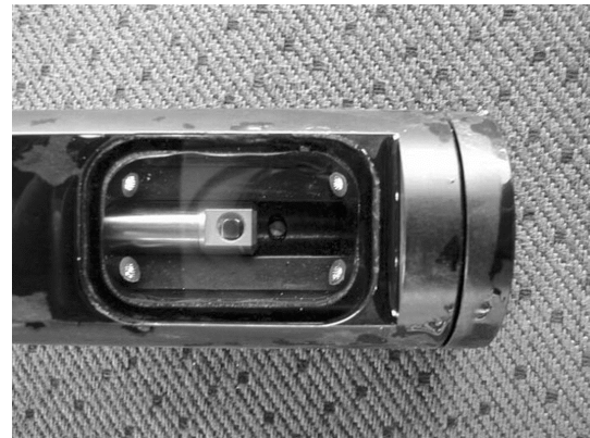
Figure 9.7 Rigid endoscope for subsoil observation. The endoscope is inserted into a protection tube containing the illumination fibers, which can be seen at the corners of the glass window.
