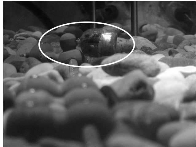
Figure 9.11 Photo of sensor above the gravel layer at y/d_{mD} = 1.0
