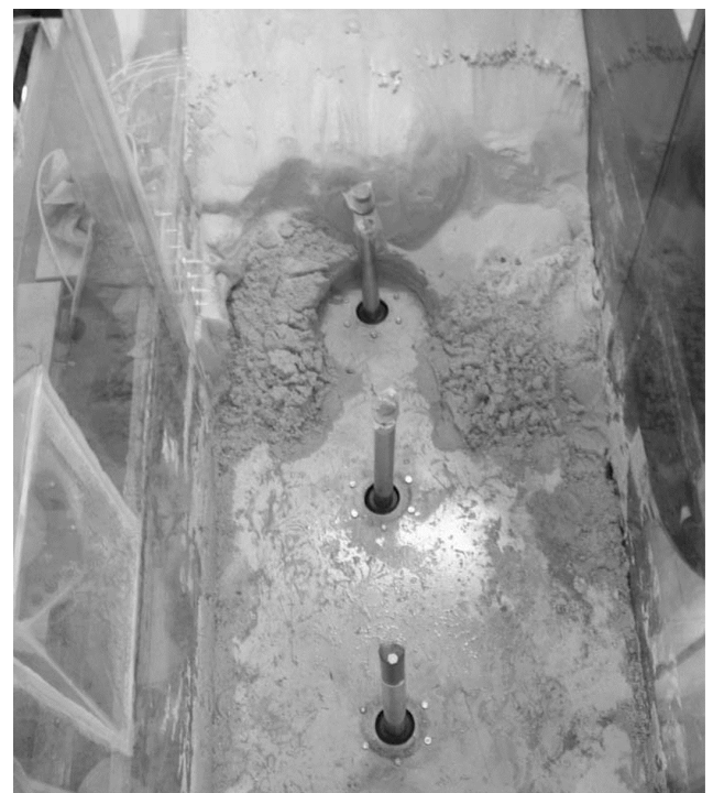
Figure 9.8 Rigid endoscopes inserted into the flume from below to observe motion of sand grains.
