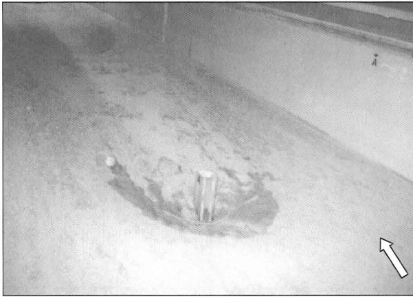
Figure 4. Scour hole resulting from Test 007_02A after 8 hours of testing at 1.0 V_c .
