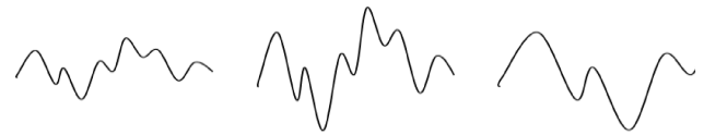
Figure 3. 2D-sketch of rock peaks (left: original, center: scaled in vertical direction (a), right: scaled in vertical and horizontal direction (b))
