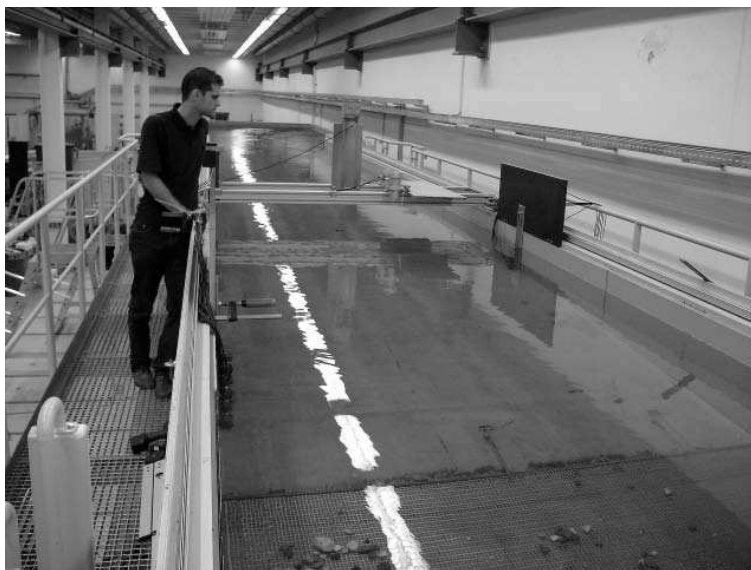
Figure 4 Lab test at the University of Kassel with 6-path installation
