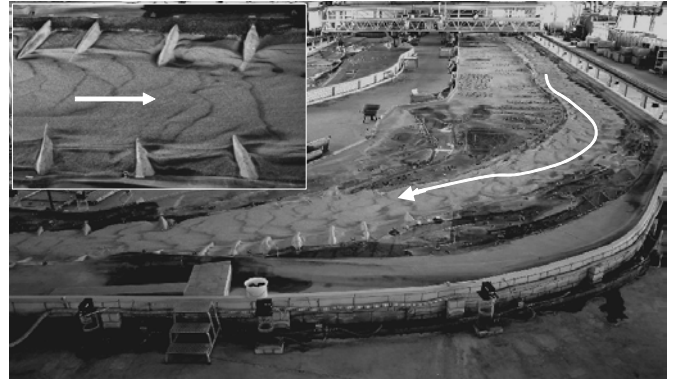
Figure 1. View of the model and detailed photograph of bed forms and training structures.
