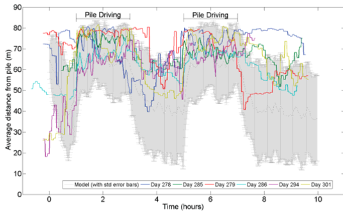
Figure 9: Measured (coloured lines) and modelled (grey error bars) distances of fish from pile during piling at the shallow end of the dock. Periods of pile driving are indicated.
