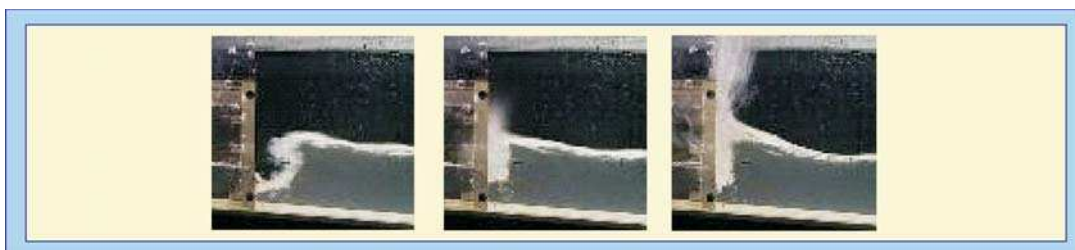
Fig. 7.4: An impulsive (breaking) wave at a vertical wall, resulting in an impulsive (violent) overtopping condition
