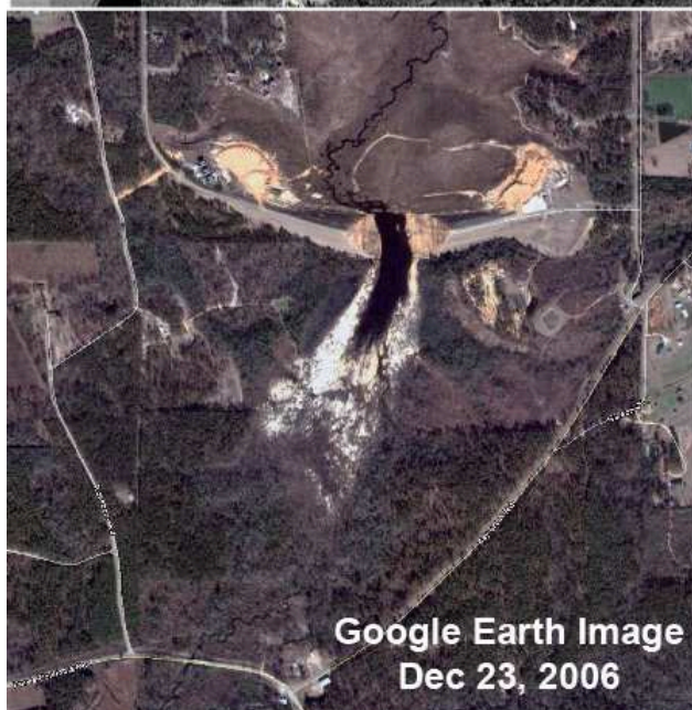
Figure 1. Satellite images of the Big Bay Dam before and after the failure. The scar left by the flood waters is clearly visible in the image below.
