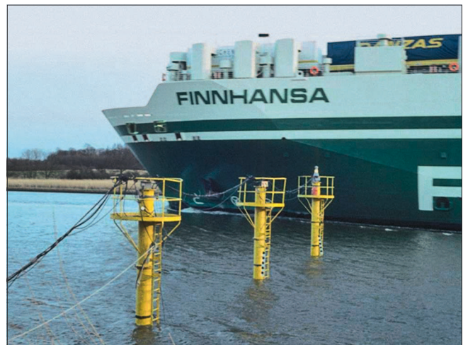
Bild 2: Messkonfiguration zur Erfassung der schiffserzeugten Belastungen an der Trave (BAW, 1996) Figure 2: Measurement configuration to determine ship-induced loads at the river Trave (BAW, 1996)
