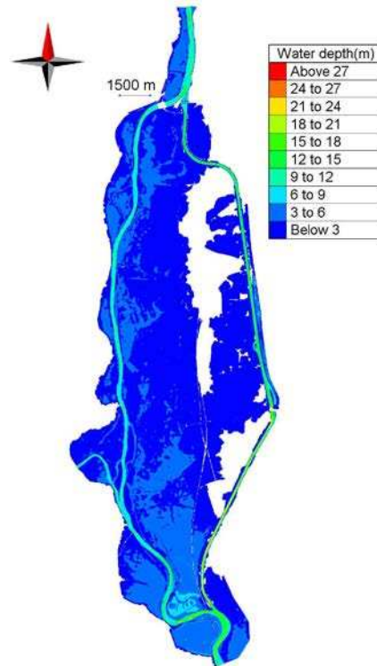
Figure 8. Map of the maximum water depths in case of extreme flood within Donzère-Mondragon developments.
