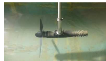
Figure 10. Photo of the 1/30th scale turbine used in the LNHE experiments
