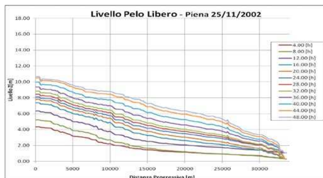
Figure 13. Profiles of the levels along Piave River between Zenson and Cortellazzo, detected, with an interval of 4 [h], since the beginning of the simulation November 24th, 2002 at 24 [h]. It may be noted that, according to the realised hydrodynamic finite element model, the maximum level of the flood is equal to 10.68 [m] at Zenson 48 [h] from the beginning of the simulation. It can be seen that the levels decrease sharply only near the mouth, even downstream of Cavetta channel placed at only 1300 [m] from the sea mouth of Piave river.
