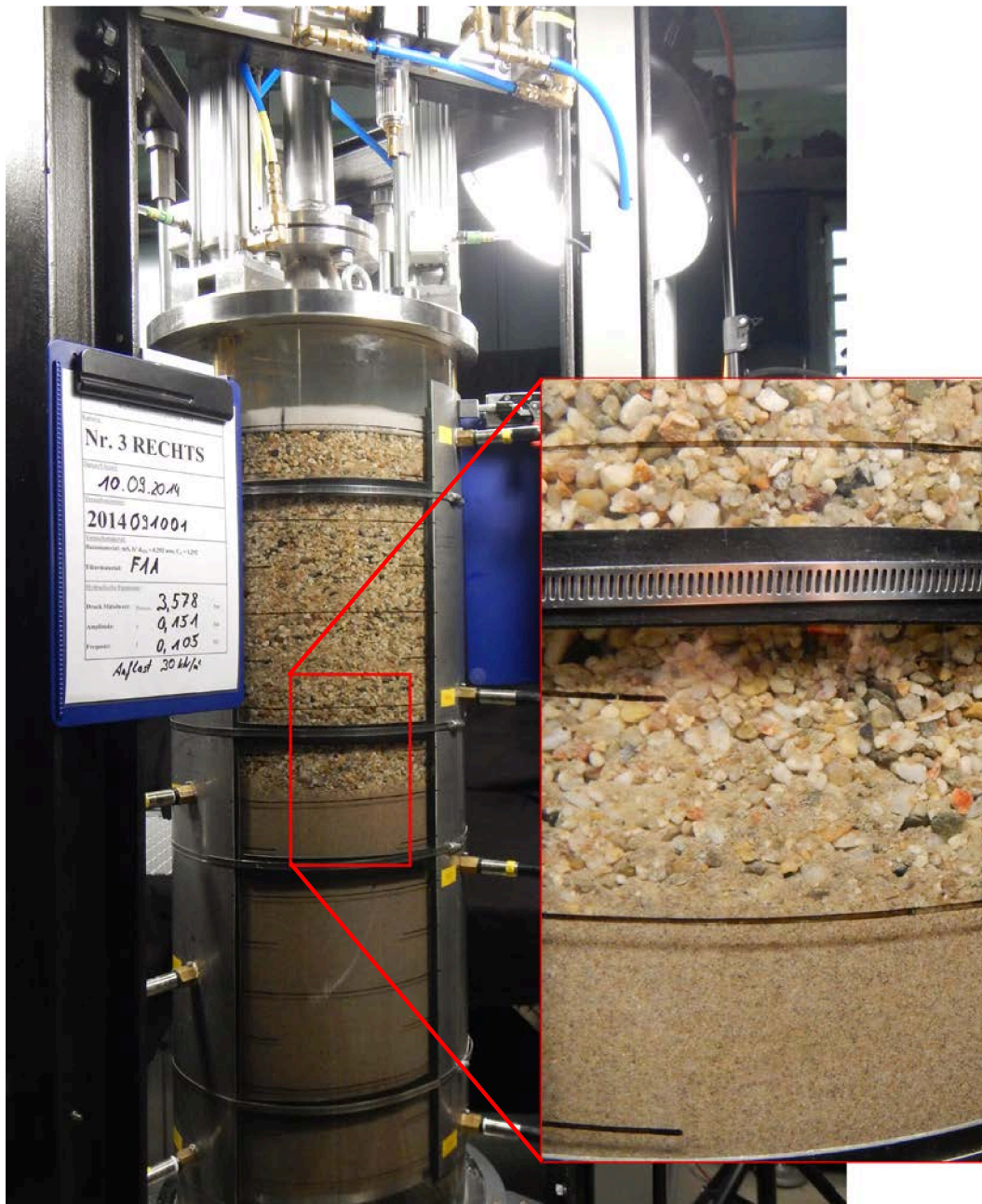
Figure 5. Test cell of the oscillatory flow facility with detail of the layer interface of filter type 1a
