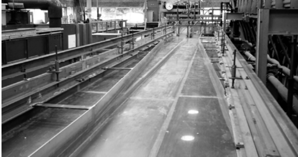
Figure 2. Photograph of the University of Birmingham's experimental flume with a skewed geometry
