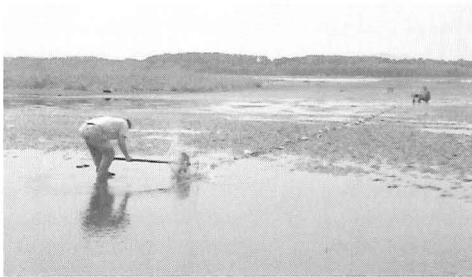
(b) Triggering of Rayleigh waves using a wooden hammer (array A)
