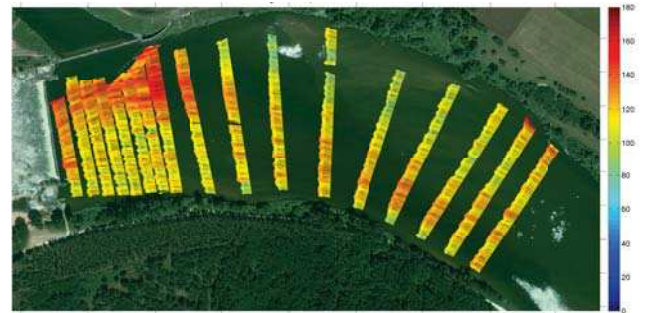
Fig. 5: Depth averaged velocities measured in the Loire River (in cm/s)
