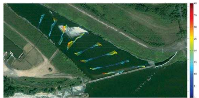
Fig. 6: Depth averaged velocities measured in the adjacent channel (in cm/s)
