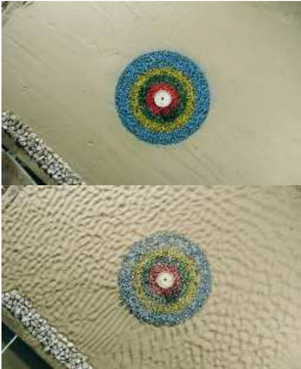
Figure 10. Scour Protection Design C before (top) and after (below) SP Test 10.
