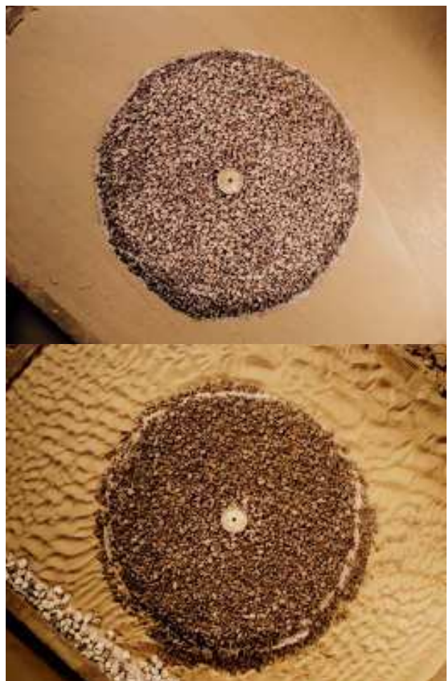
Figure 8. Scour protection Design B before SP Test 4 (top) and after SP Test 5 (below)
