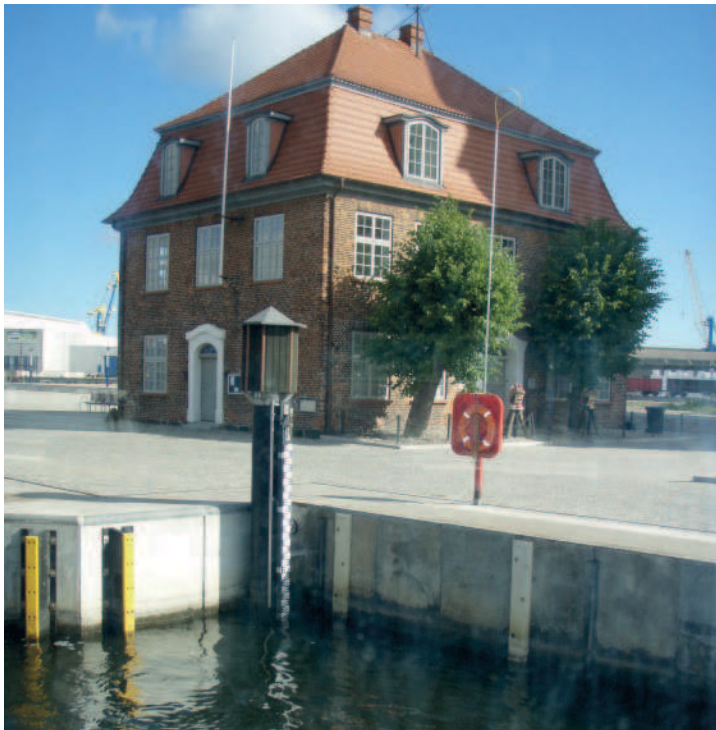
Figure 3: Modern gauge equipment, which is indicated by the smallness of the gauge house, at “Wismar Baumhaus” provides high resolution time series of water levels (photo: Seiß, 2009).
