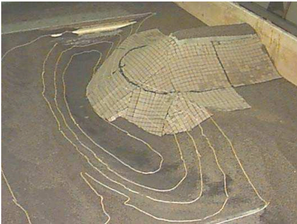
Figure 11 – Typical scour hole development for cable-tied block protection (Test 5), viewed from downstream. In this test, the protection was deemed not to have failed
