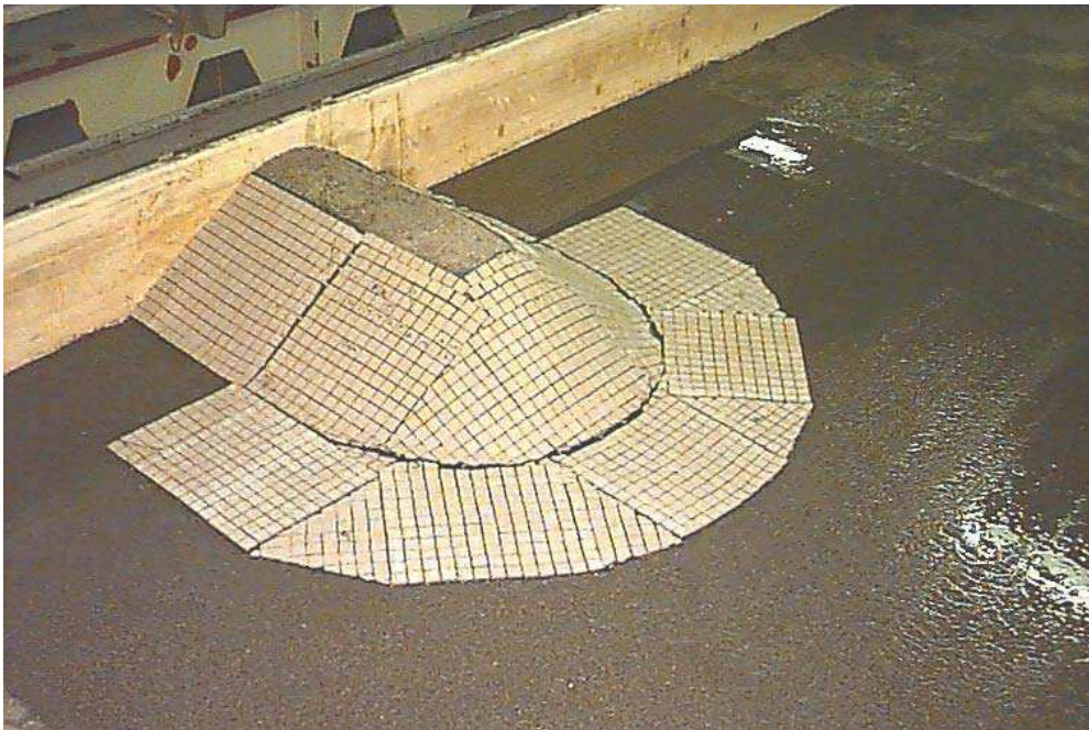
Figure 7 – The standard apron used in all cable-tied block tests
