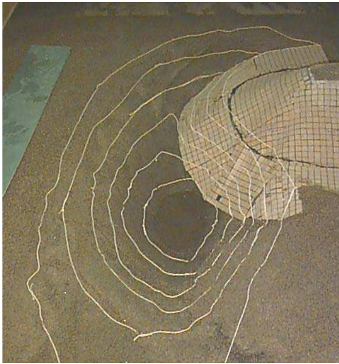
Figure 10 – Scour hole development for Test 4 using cable-tied blocks, with V/V_c = 0.66 , viewed from downstream
