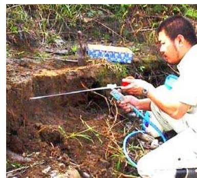
Photo.1 Situation of the jet experiment for river bank.
