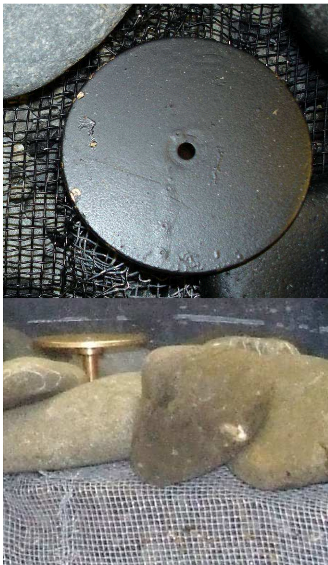
Figure 4. Top view and side view showing the mesh to prevent entrainment of smaller, underlying stones. Note: some surface stones have been removed for clarity.
