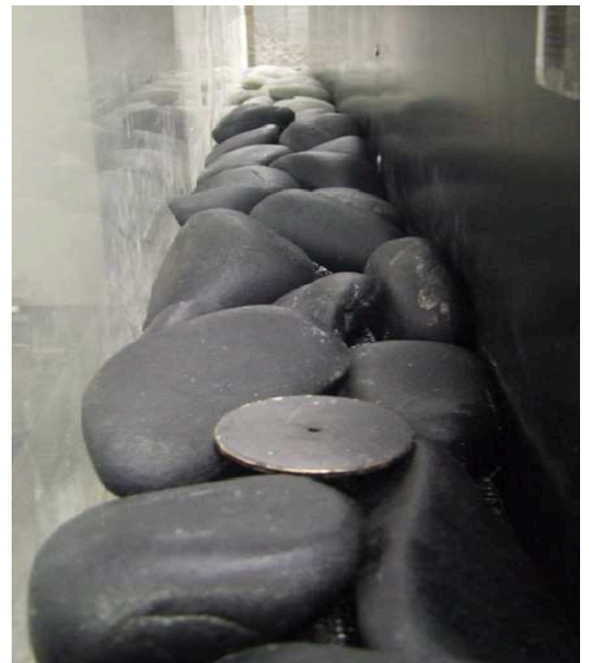
Figure 3. Typical bed configuration showing sensor plate.
