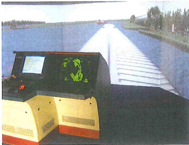
Fig. 4: View from Simulator Bridge 2 during a trail of the Pusher tug-barge system with control console containing ENC and radar image during an encounter situation with coaster
