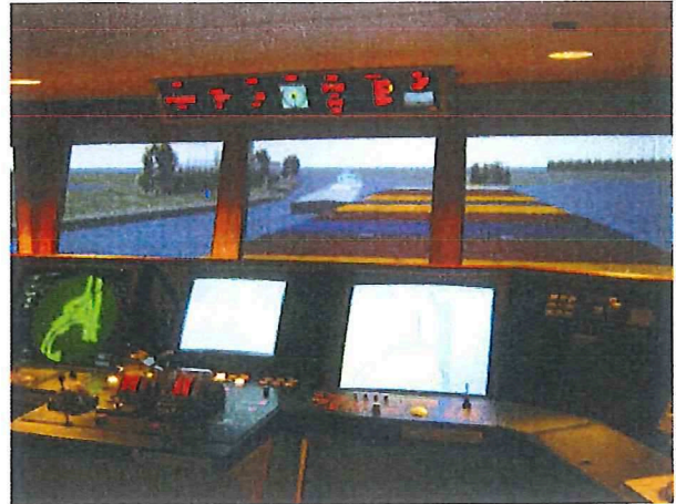
Fig. 5: View from Simulator Bridge 1 (loaded coaster) during an encounter situation with another pusher tug-barge system
