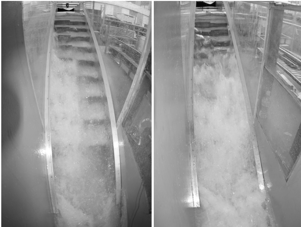
Figure 4. Three-dimensional flow down the in-line and staggered configurations of flat and pooled steps - Left: in-line configuration, Q = 0.098 \text{ m}^3/\text{s} , d_c/h = 1.54 , Re = 7.6 \times 10^5 ; Right: staggered configuration, Q = 0.090 \text{ m}^3/\text{s} , d_c/h = 1.45 , Re = 6.9 \times 10^5
