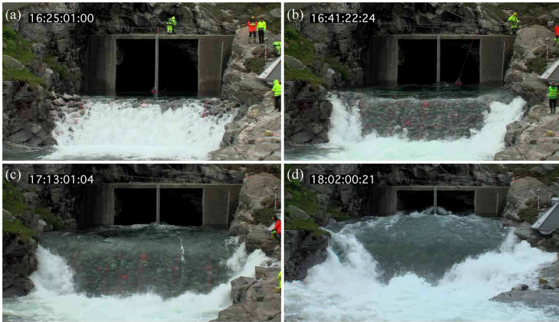
Figure 6. Picture series of F15P2: (a) nappe flow with q = 0.5 \text{ m}^2\text{s}^{-1} ( F_s = 0.6 ); (b) skimming flow with q = 1.6 \text{ m}^2\text{s}^{-1} ( F_s = 2.3 ); (c) skimming flow with still sound flow conditions upstream of the test dam at q = 3.9 \text{ m}^2\text{s}^{-1} ( F_s = 5.5 ); and (d) skimming flow in the centre part of the tests dam at q = 7.5 \text{ m}^2\text{s}^{-1} ( F_s = 10.7 ). The flow upstream of the test dam is uneven due to the inflow conditions and the high discharge of Q = 90 \text{ m}^3\text{s}^{-1} . The coloured stone in the top containing D1 is missing because it was eroded at q_s = 6.3 \text{ m}^2\text{s}^{-1} ( F_{s,s} = 8.9 ). (Video: S. R. Skilnand).
