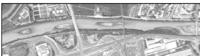
Figure 1. Alternate bars in the River Adige, at Ponte Adige (Italy). Flow from right to left. Google Earth image.
