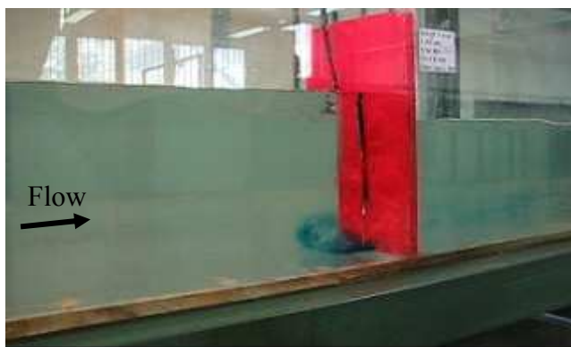
Figure 6. Flow visualization at the tip of straight groyne.
