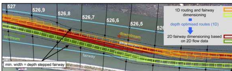
Swept areas from PeTra1D and PeTra2D calculations of vessels driving upstream and downstream and additional safety distances, resulting in the "Depth stepped fairway".
